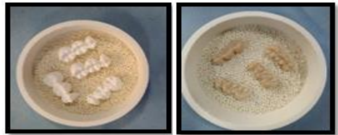
Figure 11: Before and after sintering
