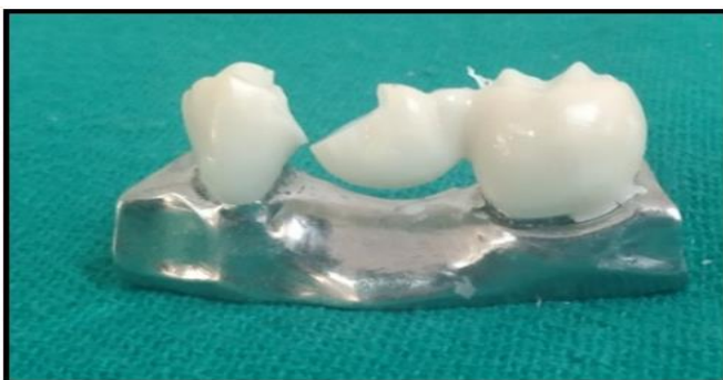
Figure 14: Fractured prosthesis after UTM testing.
