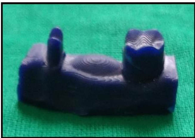
Figure 6: wax pattern attached to crucible former
