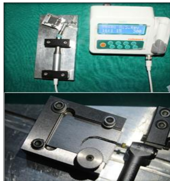
Figure 3: Rotary file with handpiece and cyclic fatigue testing device
